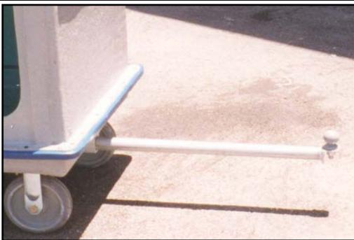
Towing mechanism shown here , fully extended from under cart for hook up. It will be hidden under cart, when cart is in service.
